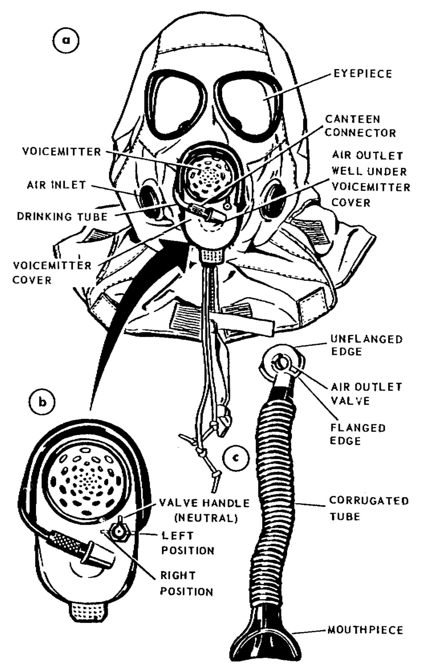
Figure 11-2. M17A1 Field Protective Mask and M1 Resuscitation Tube.
